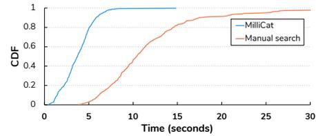
Figure 5: CDF of image usage process latency for MilliCat and manual image search.
